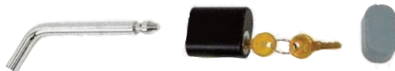
Receiver Lock Pins Two sizes to fit most receiver-type hitches. 66274 1/2" Ø, 2-1/2" usable length, 5500 lbs. Tensile strength 66275 5/8" Ø, 3" usable length, 8800 lbs. Tensile strength
