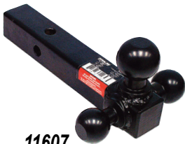
11607 1-7/8" TW 350 lb. GTW 3500 lb. 2" TW 600 lb. GTW 6000 lb. 2-5/16" TW 1000 lb. GTW 10000 lb.
